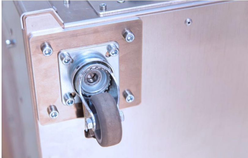
Fig. 5 Assembly of the floor rollers
