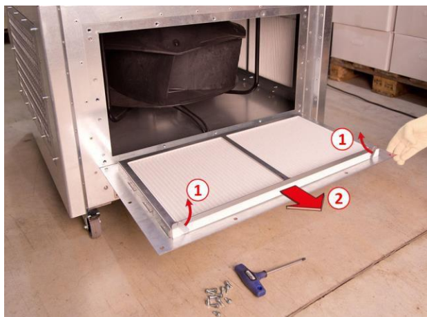
Fig. 12 Removing the blow-out damper
