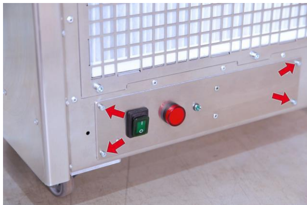
Fig. 14 Loosening the control unit screws
